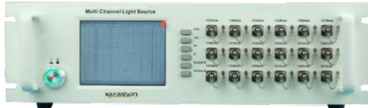
**Maxwellon TF-2304 series Bench Top Multi-functional Stable Light Source**, with DFB laser as emitter source, integrated with automatic temperature control (ATC), automatic power control (APC), and RS232C communication control. It supports 6/8/10/12/18 channel stable light source. Typical application wavelength of CWDM is 1270nm ~1610nm or 1271nm ~ 1611nm; DWDM wavelength follows ITU-T standards; Other wavelength is available to custom-made.
