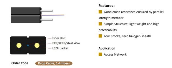
Maxwellon TF-3701 series FTTH Drop Cable (without self-supporting wire) construction is that the optical fiber unit is positioned in the centre; Two parallel strength members are placed at the two sides; The cable is completed with a LSZH sheath.
