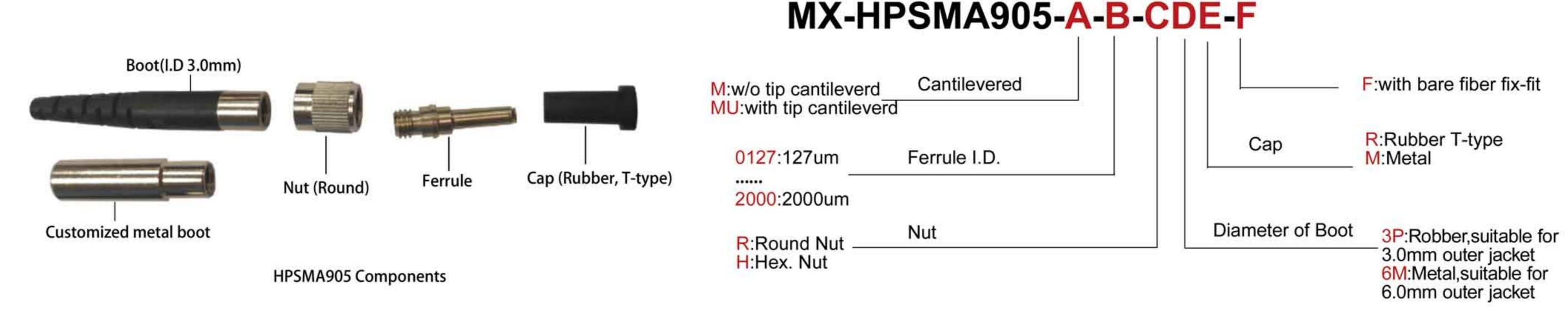
For example: MX-HPSMA905-M-0610-R3PR-F HPSMA905 Connector, Cupronickel ferrule, Without tip cantileverd, Ferrule I.D.610um, Round Nut, Rubber T-type Cap, Rubber boot, Suitable for 3.0mm outer jacket, With bare fiber fix-fit.
