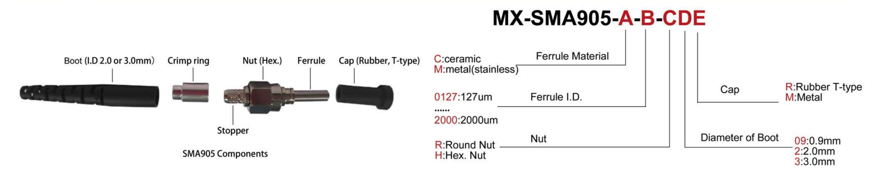
For example: MX-SMA905-M-0610-R2R SMA905 Connector, Stainless Ferrule, Ferrule I.D.610um, Round Nut, 2.0mm Boot, Rubber T-type Cap
