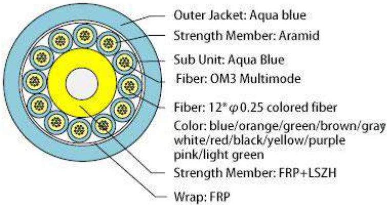
144 core trunk cable structure
